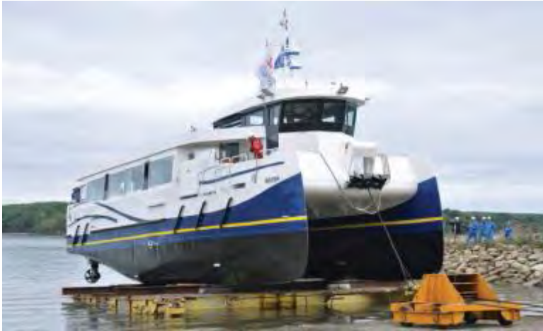
Ar Vag Tredan super-capacitor driven ferry
