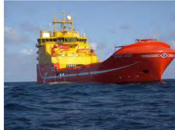
Eidesvik offshore support ship Viking Lady first commercial fuel cell hybrid propulsion
